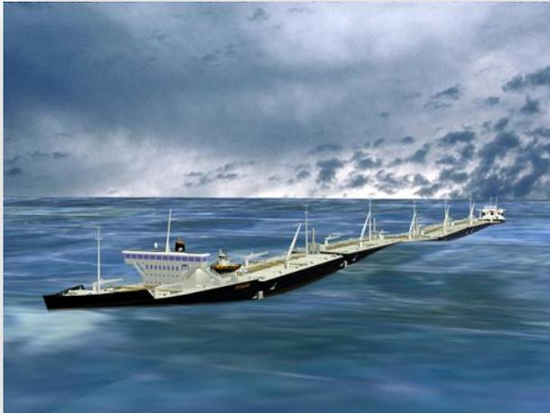
One of three designed models fits the Great Lakes. A big plus--no ballast water is needed so no new invasive species issues! The individual cargo units can carry a diversity of cargo and be disconnected to leave or take units at various ports and allow the snake to be broken into smaller pieces to fit through the existing locks of the St. Lawrence Seaway system. Cost savings are projected in both construction and operation compared to traditional lake freighters.
